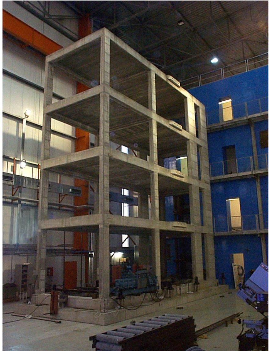
**Figure 3. Full-scale RC frame in preparation for pseudo-dynamic testing at the ELSA reaction wall facility**
