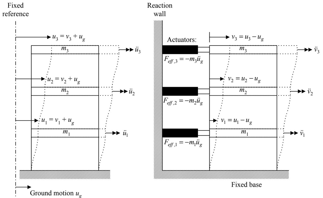
**Figure 6. Effective force test method**
