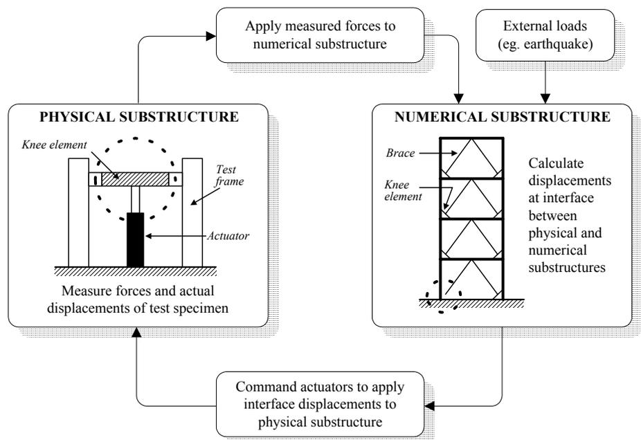
Figure 5. Control loop for real-time substructure testing
