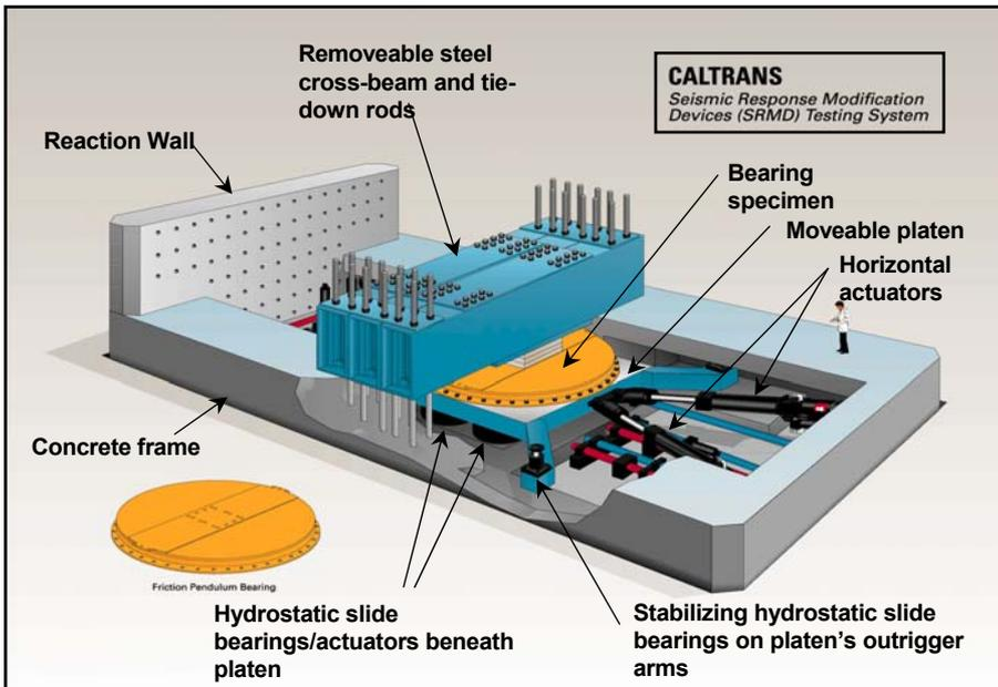
Figure 4. Schematic of the Caltrans SRMD test facility
