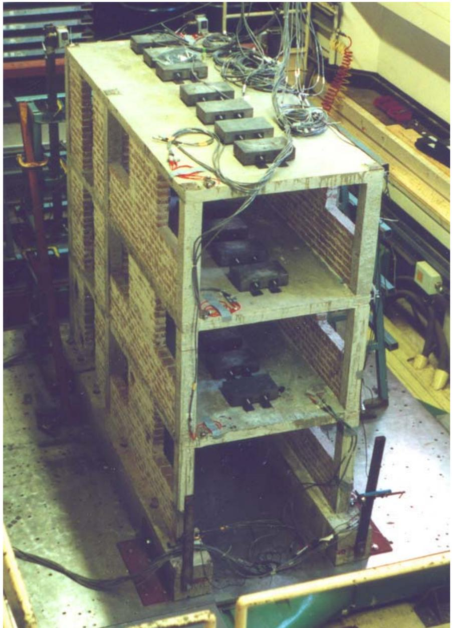
**Figure 1. Model of a concrete frame with masonry infills on the Bristol shaking table**
