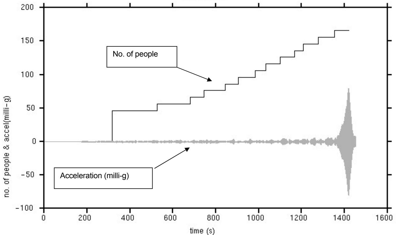
**Figure 2. Variation of number of walkers and lateral acceleration of the bridge with time, showing the sudden instability when a critical number of walkers is reached**
