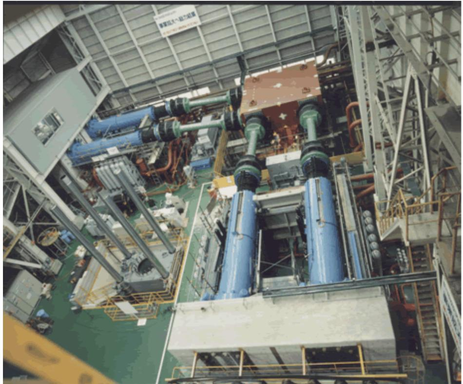
**Figure 2. Commissioning test of 450 tonne actuators for the NIED 1200 tonne shaking table**
