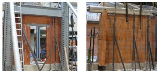
Figure 3. Illustration of (left) a simple wall with an opening (A 3/A 5) and (right) a T-shaped wall (C 1-3)
