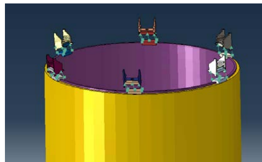
(b) 10% Bulk loss of grout (with TP-grout debonding)-No ovalisation/buckling of the pile as it is stiffened due to bonding with the grout
