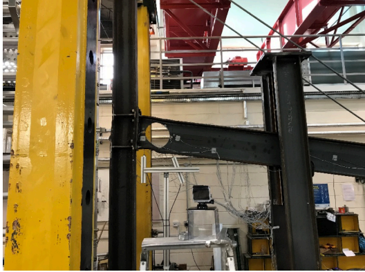
Figure 12. Ultimate failure of RWS_1
