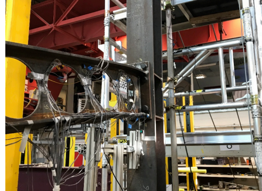
Figure 13. Ultimate failure of RWS_2
