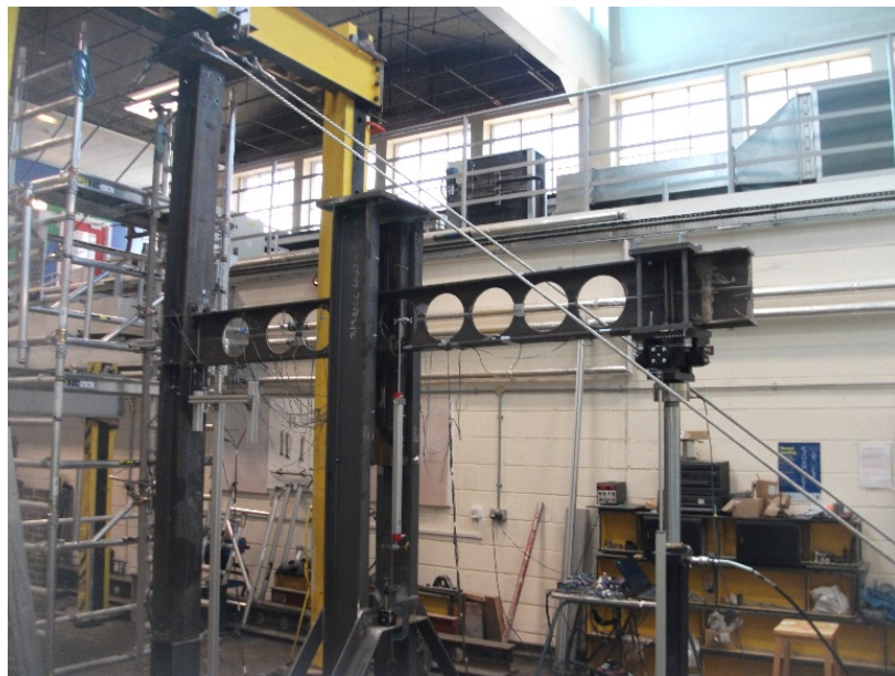
Figure 2. General arrangement of test specimen (RWS_3)
