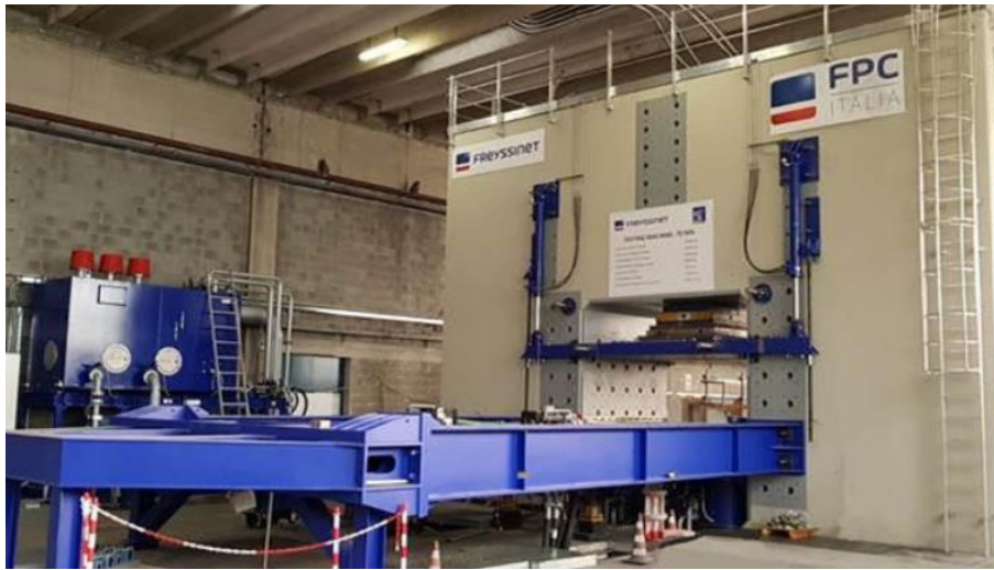
Figure 10. Test equipment: 70MN vertical capacity
