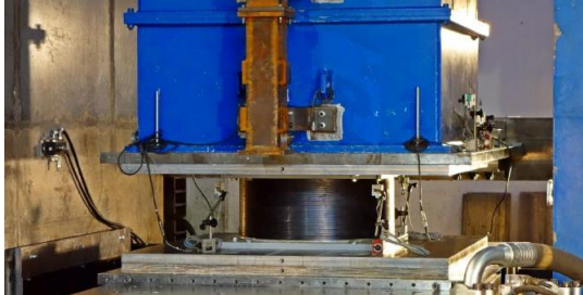
Figure 17. Marmara: Test on LRB at Eucentre Figure 18. Marmara: Test on NTm at ISOLAB
