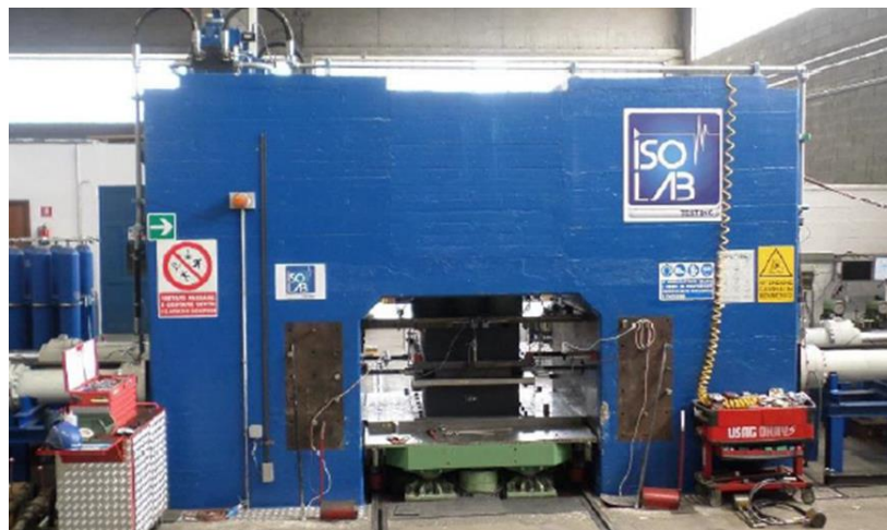
Figure 5. Test equipment: 50MN vertical capacity
