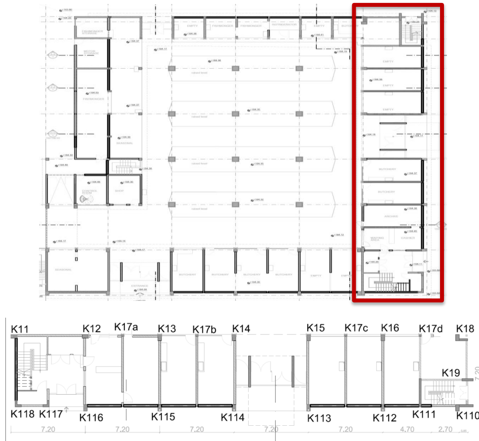
Figure 2. First floor and denomination of frame members.
