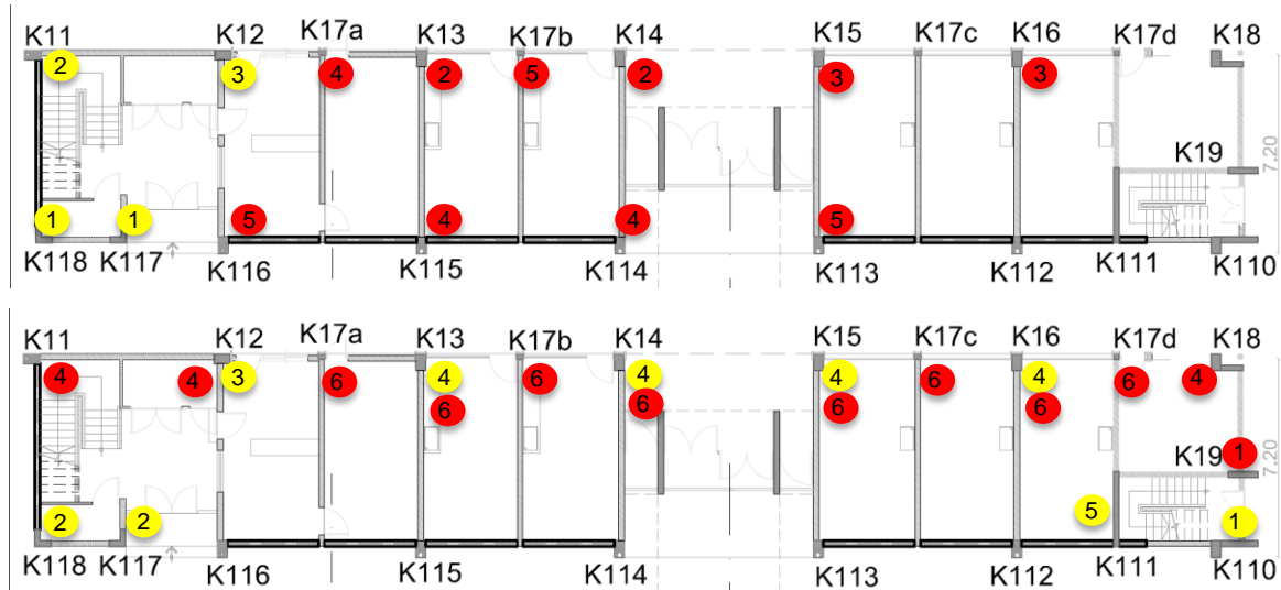
Figure 6. Displacement control pushover progressive failures in Y (top) and X-directions (below)
