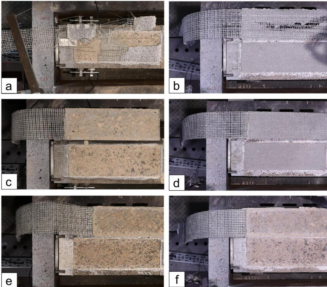
Figure 4 Mode of failure of different specimens from (a) Series SB-M41, (b) Series SB-M81, (c) Series SB-M42, (d) Series SB-M82, (e) Series SB-M43, and (f) Series SB-M83
