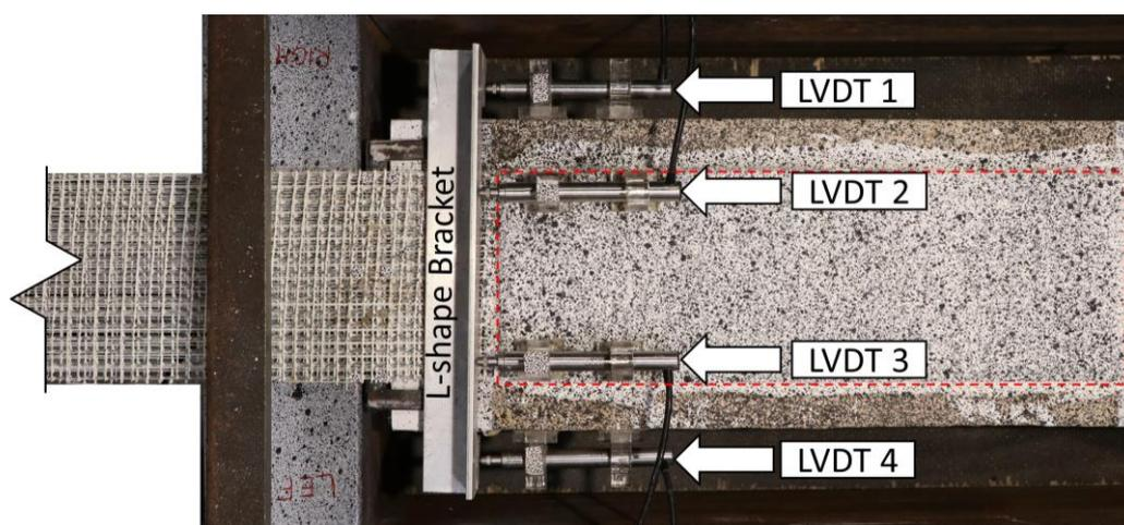
Figure 1 Instrumentation of the shear bond test
