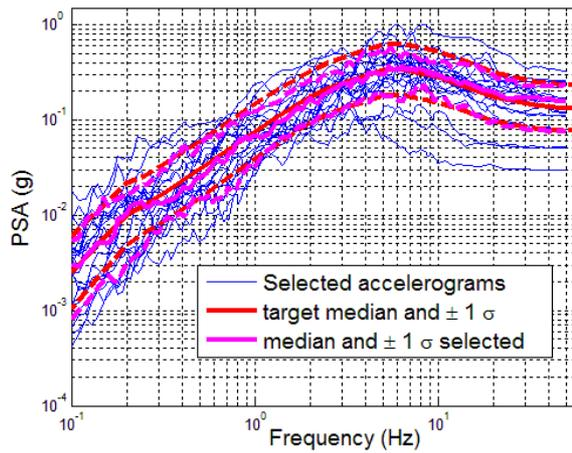
Figure 1. Response spectra of selected accelerograms using the Jayaram, Lin & Baker 2011 algorithm.
