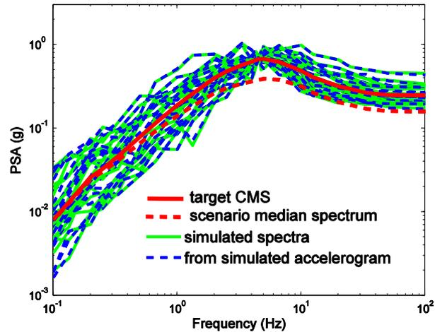
Figure 6. Response spectra of simulated accelerograms compared to target (red)
