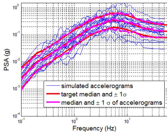
Figure 2. Response spectra of simulated accelerograms using the Zentner 2014 algorithm.
