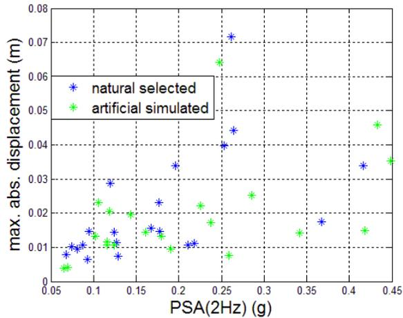
Figure 5. Scatterplots of max abs displacement against PSA(2HZ) for simulated (green) and selected (blue) accelerograms.
