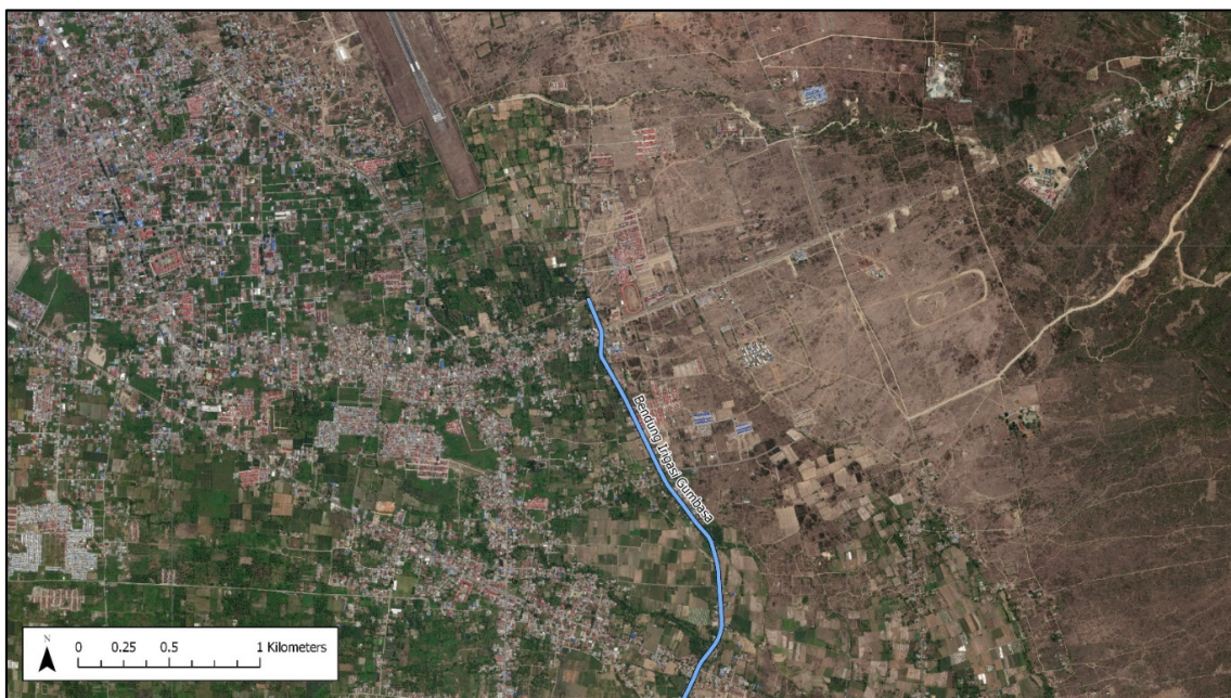
Figure 5. Difference in vegetation growth due to groundwater conditions on either side of the Bendung Irigasi Gumbasa. Green vegetation growth (left) indicates wetter ground conditions as opposed to brown land with lack of vegetation growth (right) indicating mostly dry ground.
