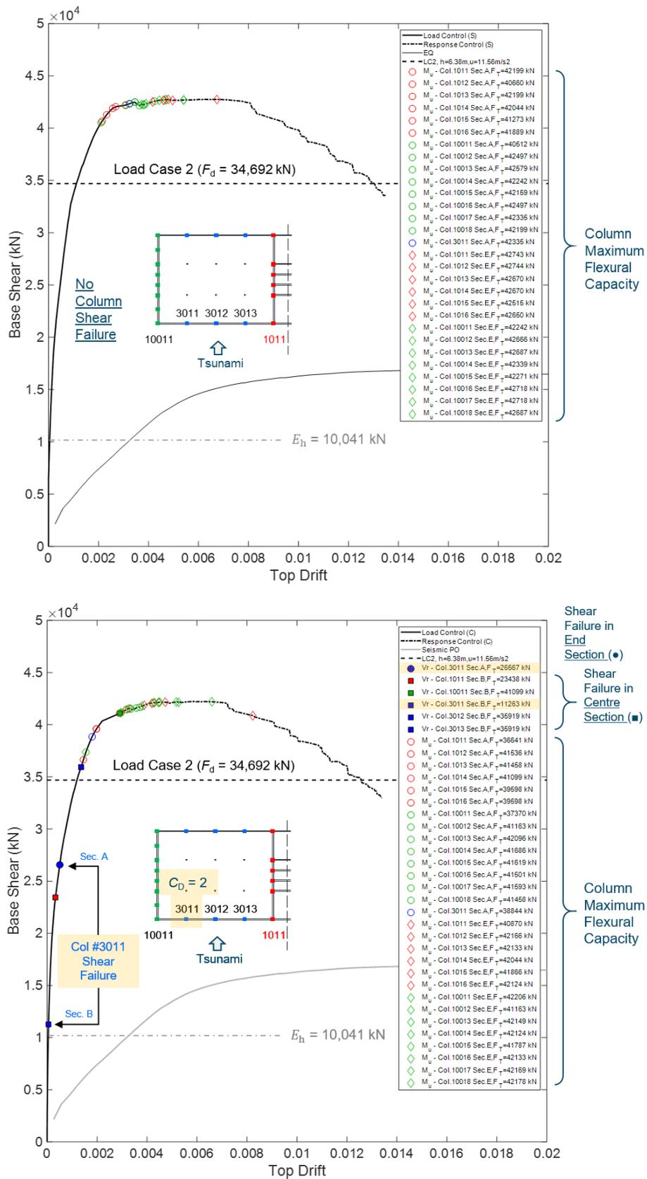
Figure 8: Base-shear-top drift curves from seismic PO and tsunami PO with load discretisation method S (top) and C (bottom), with sequence of maximum flexural capacity and shear failure attainment (for ground floor columns)
