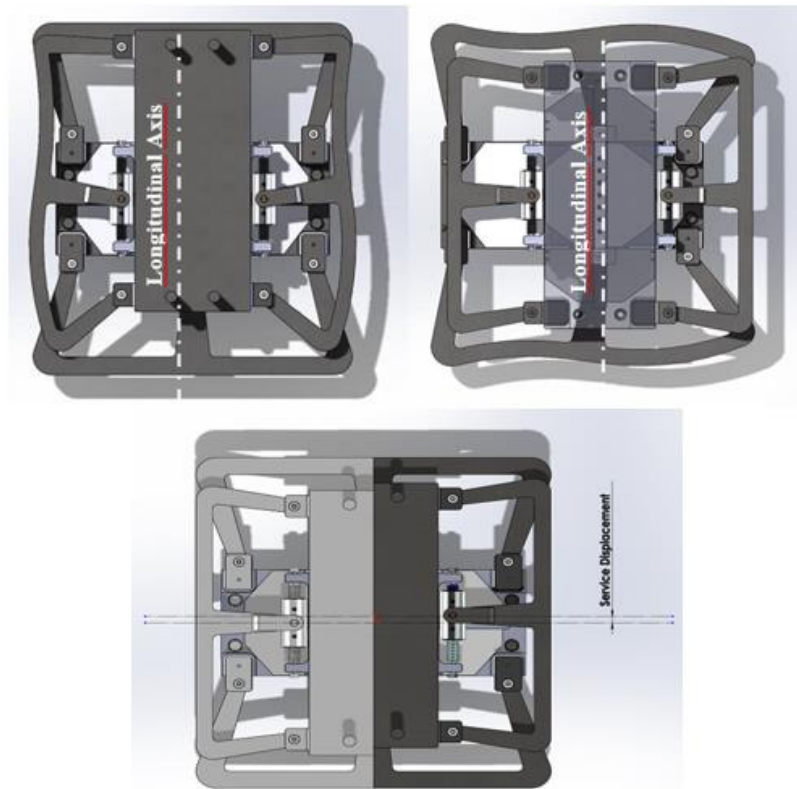
Figure 11. Longitudinal (top left) and transversal (top right) configuration in seismic condition and service configuration (bottom).
