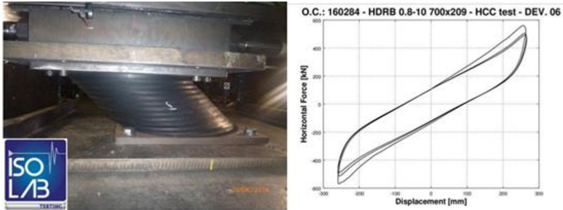
Figure 16. Testing of HDRB and associated hysteretic response.
